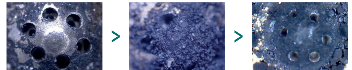
These images show the injector holes before the dirty-up phase (left), fouled after the dirty-up phase (middle) and the clean-up achieved with PROGILINE FA-G (right).
